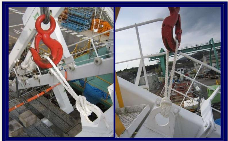
Tie both end rope rings to the eye plates as is shown in the photo. This can avoid loosening or falling of the rope during davit operation.
