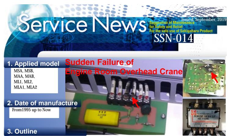
During operation of engine room crane, a trouble of hoisting motor suddenly happened and hoisting up and down became inoperative.
