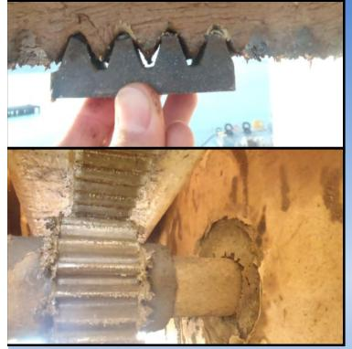
RGE-7/4 Manufactured in 2001 (Photo taken in 2014) Pinion makes only small contact with the Rack by corrosion caused by rust
