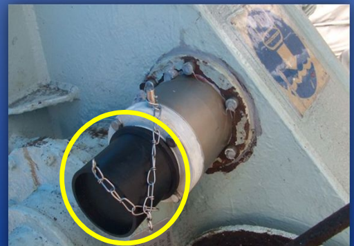
Rubber cap installed on cam clutch.
